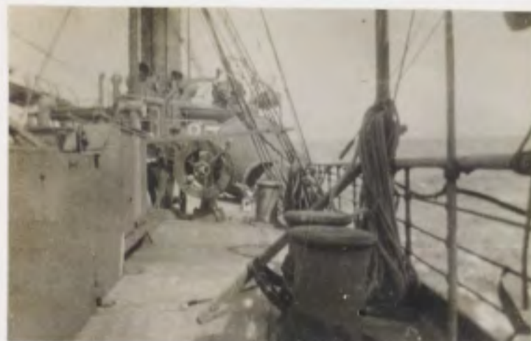
13. The measuring wire gear.
